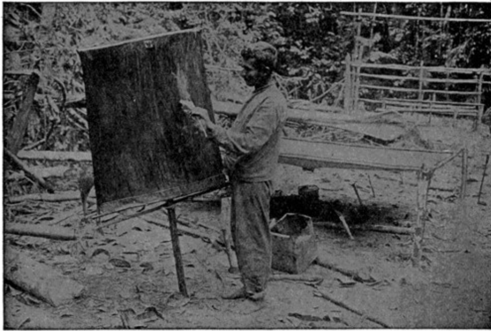
INDIAN WATERPROOFING CLOTH BY "PAINTING" IT WITH RUBBER "MILK"—BRAZIL
