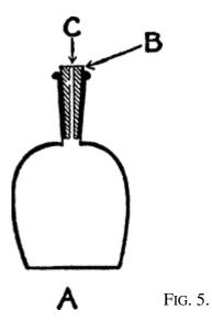
A, Flask-like Bottle; B, Indicates Ground Glass Stopper; C, Shows Hole Drilled through Stopper.
