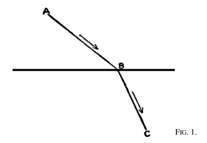
AB represents the path of light in the air and BC its path in the water.
